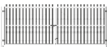
Double leaf gate Max. width up to 7500 mm Max. height up to 2600 mm
